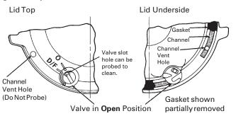
**Drip Free Mode "D/F"** - To operate in the drip free mode, rotate the valve with a screwdriver or coin so that the hole in the valve slot is aligned with the "D/F" on the lid. See Figure 3.
